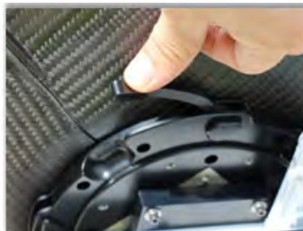
Figure 3-6: Center hub with four latches for the 4 panels
