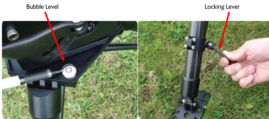
Figure 2-2. Leveling the tripod legs
