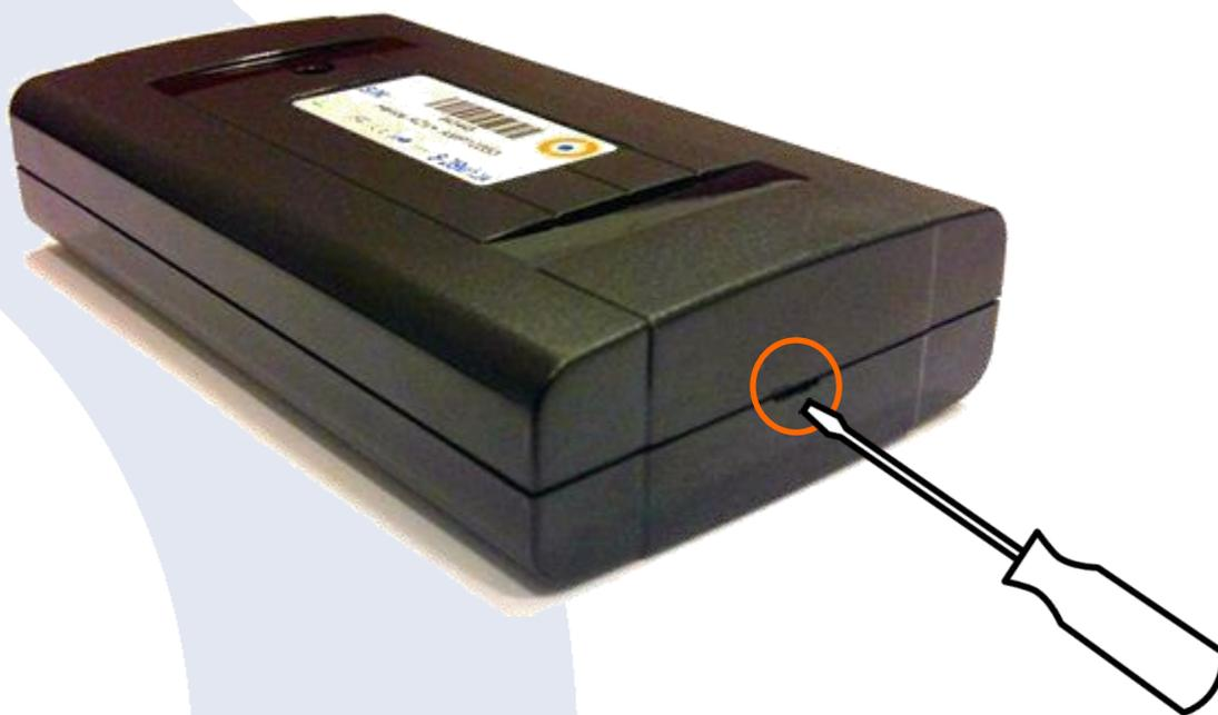
Gently push and pull back the plastic SIM card holder to release and open the SIM card slot. Raise it to an upright position.
