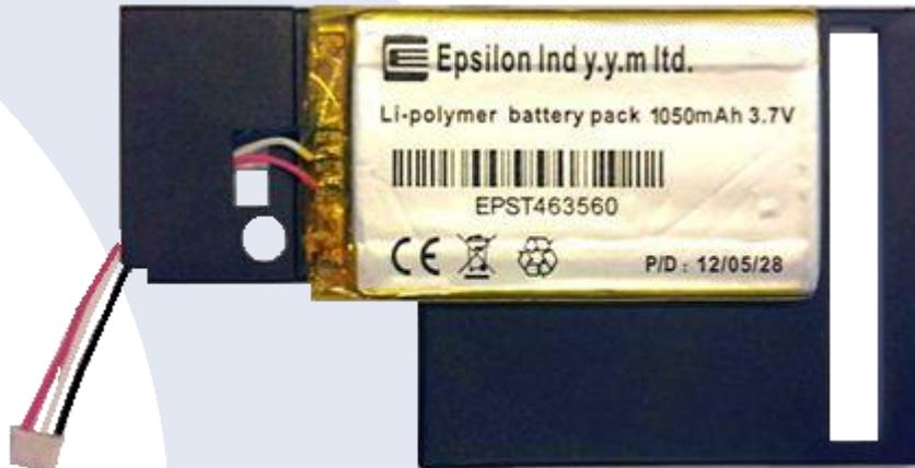
Verify that you're connecting the battery connector to the connector on the unit board correctly. The side of the battery connector with the pinholes located closer to the edge
