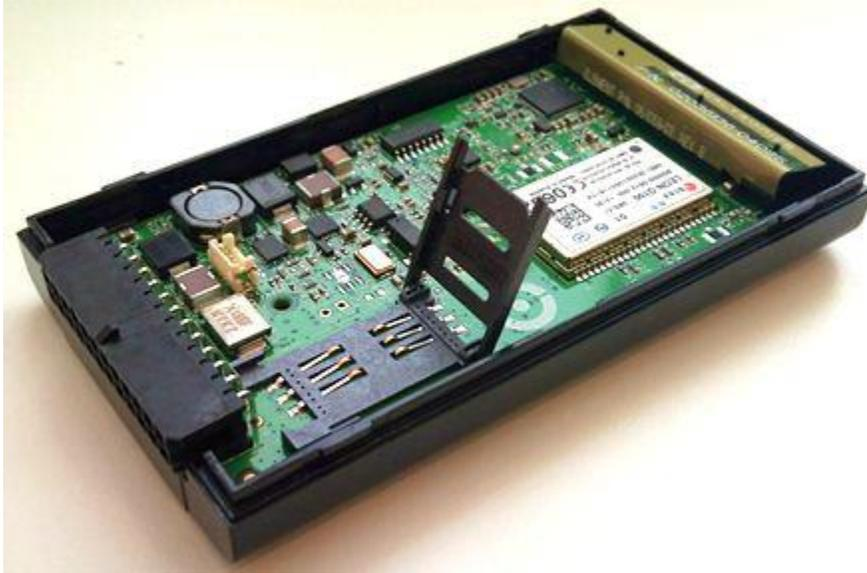
Insert the SIM card in the SIM card slot with its gold contacts facing down and its cut-off corner facing out the SIM card slot, as shown in the following image.
