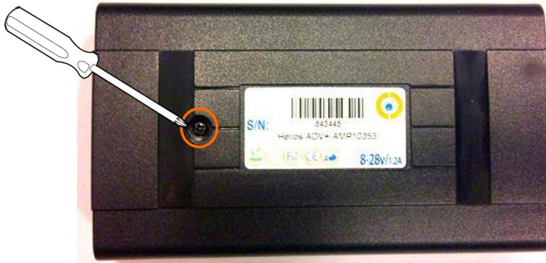
Insert a flat screwdriver in the slot between the unit covers. Carefully twist the screwdriver to lift and open the unit cover.
