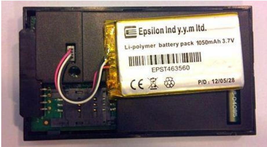
Place the bottom cover so that the battery cable is coiled around the plastic pin of the bottom cover screw.
