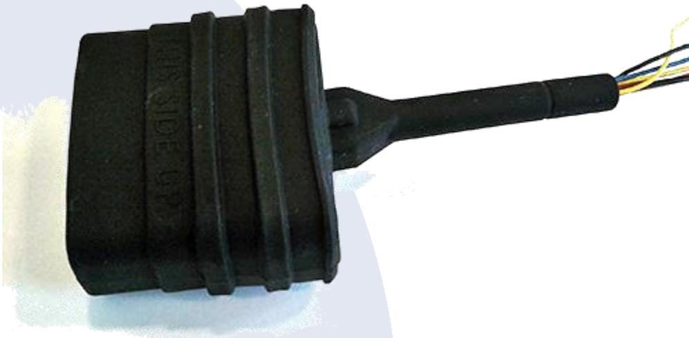
Bend the wire harness sleeve on the smaller casing part.
