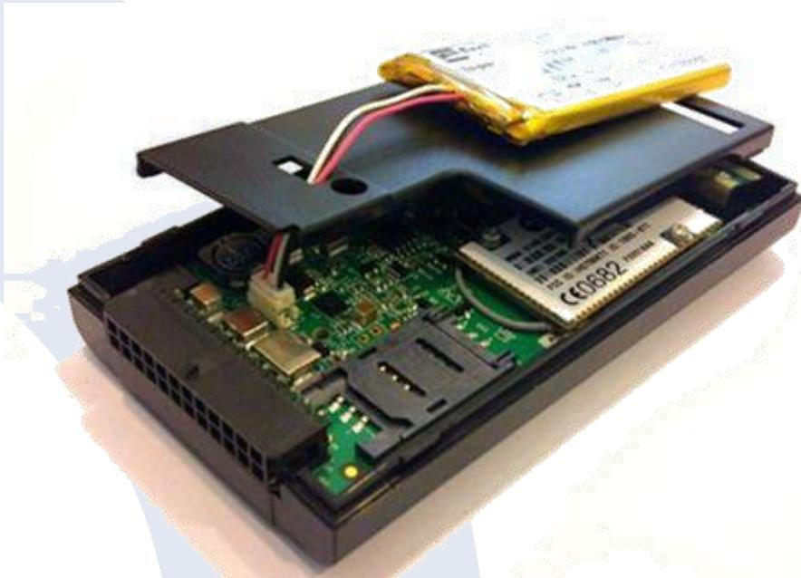
Snap the divider on the top cover and place the battery on it as shown in the following image.
