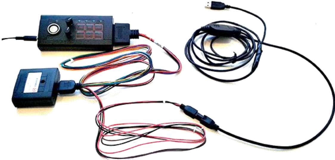
Connect the Helios TT unit to the Simulator with the 10-pin wire harness.
