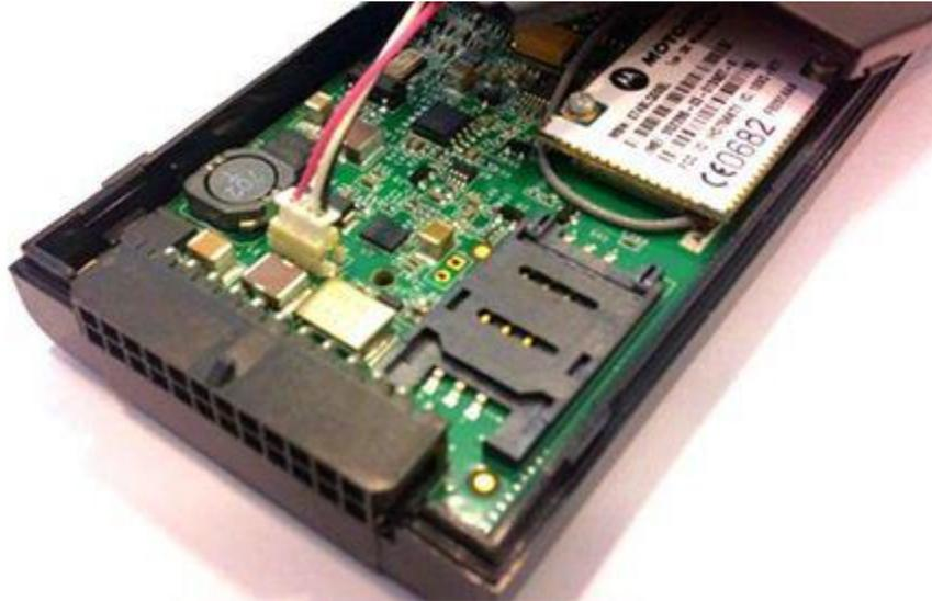
Gently push the battery connector into the connector on the unit board. If necessary, use a small flat screwdriver. Be careful, do not use excessive force!
