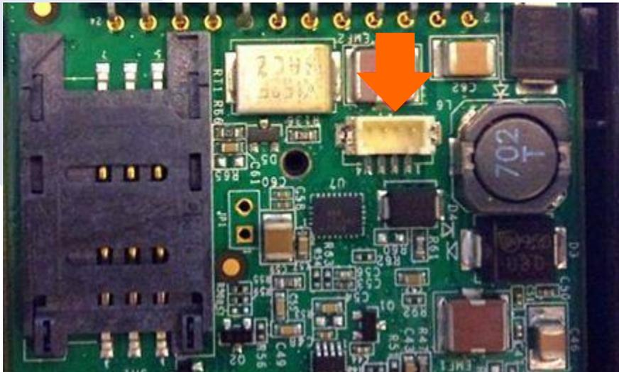
Carefully insert the battery connector into the connector on the unit board.
