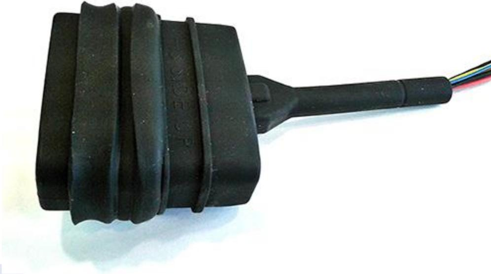
Unfold the sides of the larger part of the casing over the smaller part and pull them up as tight as possible, as shown in the image below.
