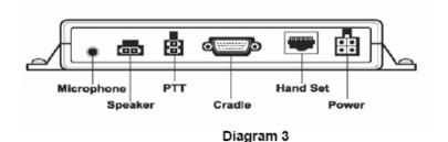
3. Route the cables out of the way to avoid physical or visual obstruction. Allow sufficient slack in the cable to the PTT so that it does not interfere with the movement of the gear lever.
