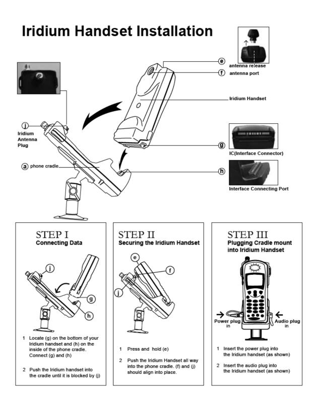
Note: If you own the 9555 version of the SatStation Standard Dock, parts h and j are located on the top portion of the 9555 cradle.
